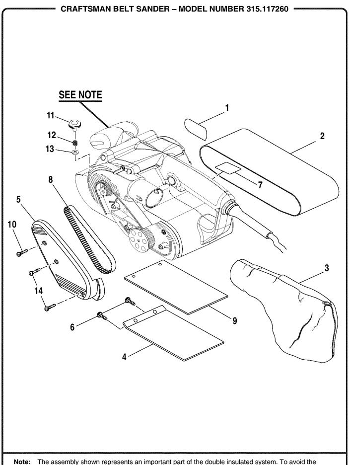
The assembly shown represents an important part of the double insulated system. To avoid the possibility of alteration or damage to the system, service should be performed by your nearest Sears repair center. Contact your nearest Sears retail store for service center information.
